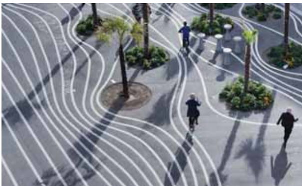
Surface treatment such as painted asphalt can be cost effective material to improve wayfinding for pedestrian.
