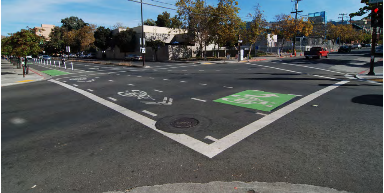
On separated bikeways, the two-stage turn box can be located in the protected buffer/parking area.
