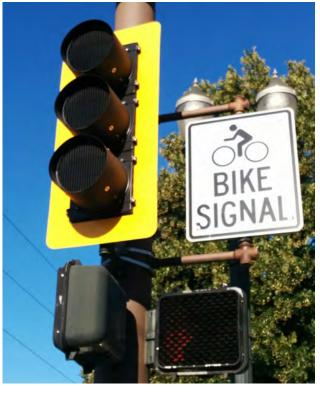
Signal louvers or visibility-limited signal faces reduce the likelihood of motorist in adjacent travel lanes mistaking the bike signal indication with a circular or arrow indication for their travel lane
