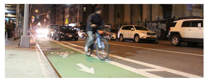
Parked cars in the image above serve as a barrier between bicyclists and the vehicle lane. Barriers could also include flexible posts, bollards, planters, or other design elements.
