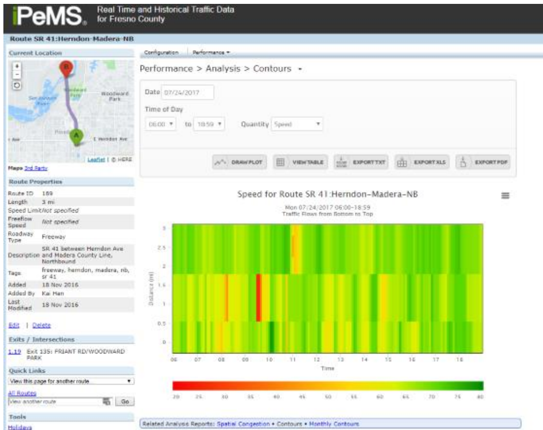
Figure 7: Example Daily Contour Plot showing average speeds along a route throughout the day
