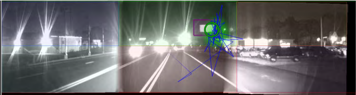
Figure 15. Heat map for the middle of a DCZ for a standard billboard at night on an arterial.
