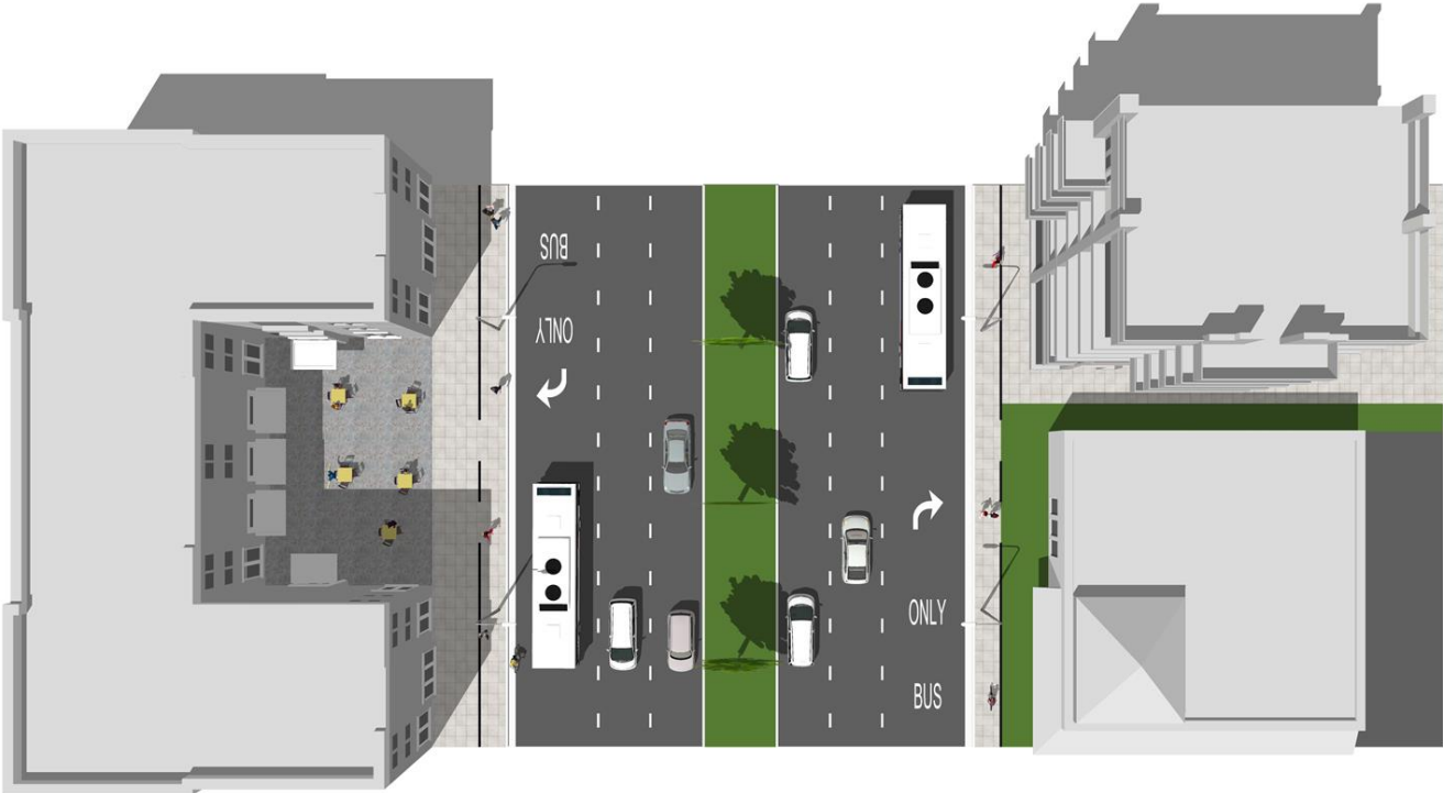
Figure 10: Alternative A aerial showing inconsistent sidewalk width
