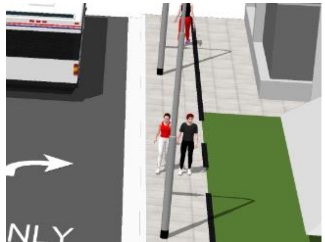
Figure 7: Existing 6' sidewalk (foreground) is still constrained, while redeveloped sidewalk (background) provides more space.
