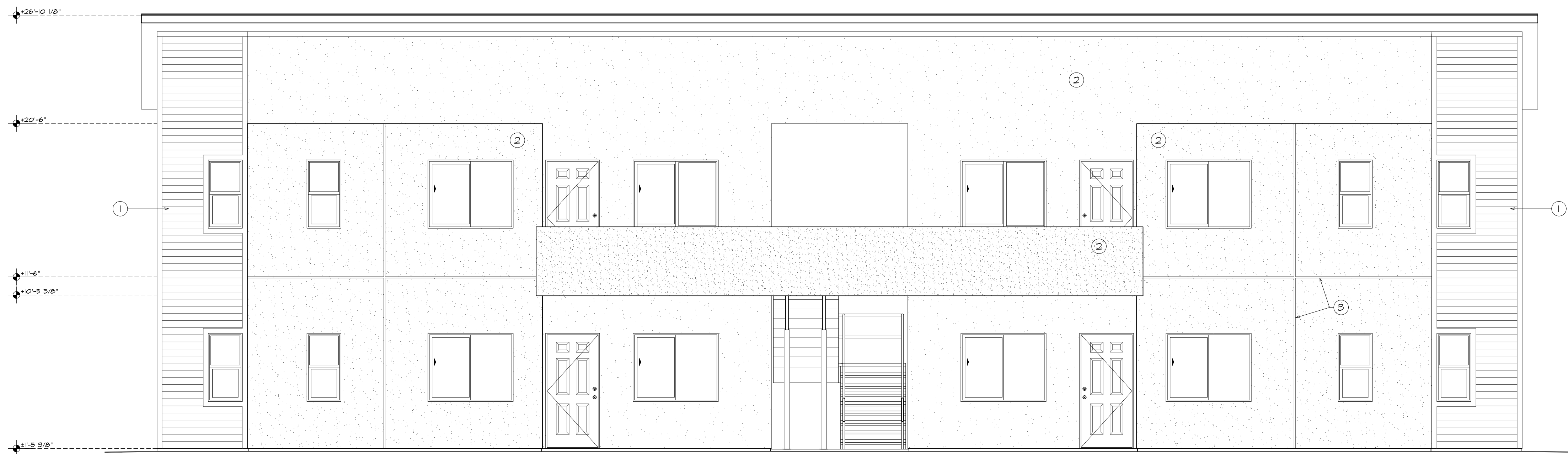
NORTH ELEVATION - BUILDING #1 SCALE: 1/4" = 1'-0"
