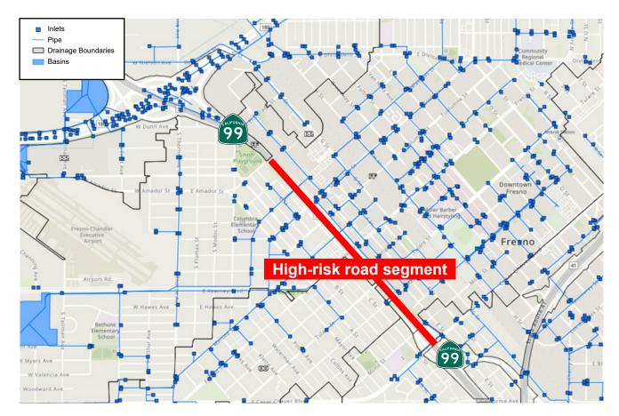
Stormwater management controls placed throughout the drainage, at the northeast end and throughout downtown Fresno, could help to mitigate the volume of runoff that enters the storm system or that flows onto this segment of SR-99. Sizing the storm system to account for larger precipitation events and flooding can help to move stormwater runoff from the street surface and into existing stormwater treatments, such as bioretention basins.
